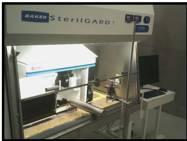
Figures 8&9 3 - 100mm Setting Plates Placed Inside Sorting Chamber For Product Protection Test
