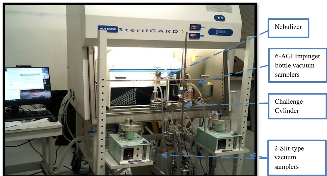
Figure 3 Personnel Protection Microbiological Test Set Up
