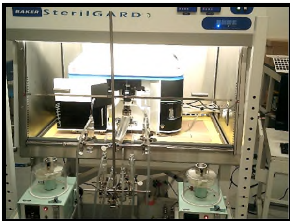
Figures 6&7 Nebulizer Placed Inside Sorting Chamber For Personnel Protection Test
