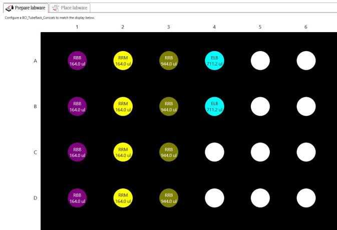
Figure 5. Guided Labware Setup indicates reagent volumes and guides the user for correct deck setup
