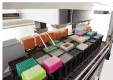
Figure 1. Biomek i7 Hybrid Genomics Workstation with optional enclosure on a Biomek Cart. 45 position deck capacity maximizes efficiency and increases walk away time.
