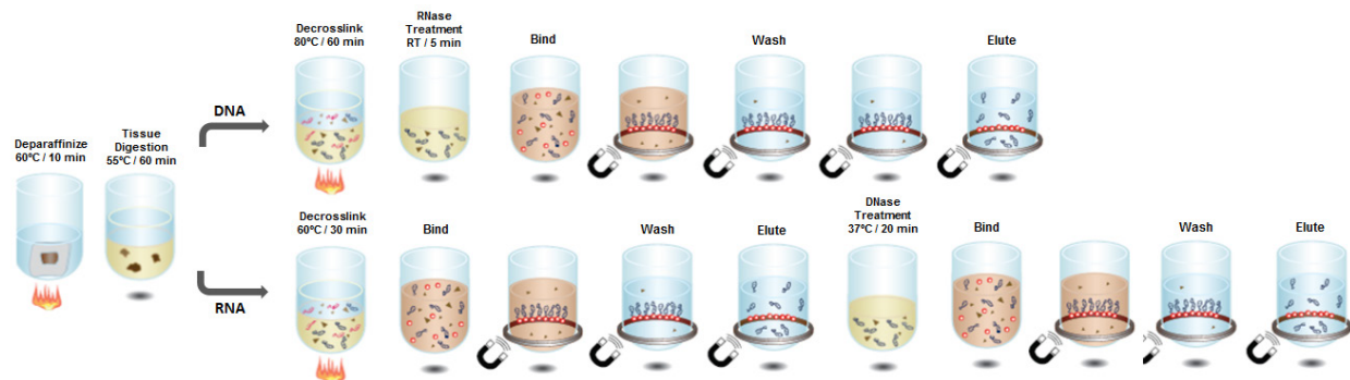
Figure 1. Process overview. Deparaffinization, lysis and decrosslinking incubation times and temperatures were modified to retrieve high quality RNA from FFPE tissues. Total nucleic acids can be isolated by dividing the samples after the lysis step (refer to text for details).
