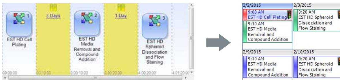
Figure 7. Automated HDP Compound Screen. The software for an automated screening system can link together the steps of the four day workflow and interleave experiments on a calendar to show instrument availability.
