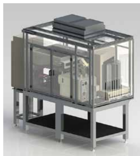
Figure 8. Automated HDP Compound Screen. A rendering of a potential HDP screening system that utilizes imaging as the primary assay. Plating, treatment, and staining could be completed using a Biomek NX ® Workstation with a 96-channel EST head while analysis is performed on an integrated ImageXpress Micro.
